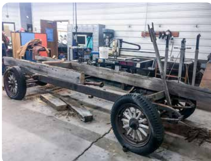
Students removed the old wood, fixed minor frame issues, and removed unnecessary parts from the hay wagon.
